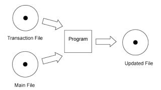
The picture shows the main file and the transaction file as input to a program. The output is a new, updated main file. The previous version of the file can be kept as backup.
