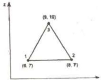
4. Calculate the element stiffness matrix and thermal force vector for the plane stress element shown in fig. The element experiences a rise of  $10^\circ\text{C}$ .
